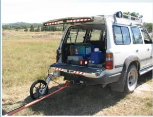
The resistivity profile below was recorded in a region in Cumbria United Kingdom which was known to have been part of an open cast mine in the 1970's and was subsequently filled and returned to farming land. The purpose of the survey was to map the extent and depths of the mine pits to help establish the bearing capacity of the ground before the proposed construction of a wind farm.
